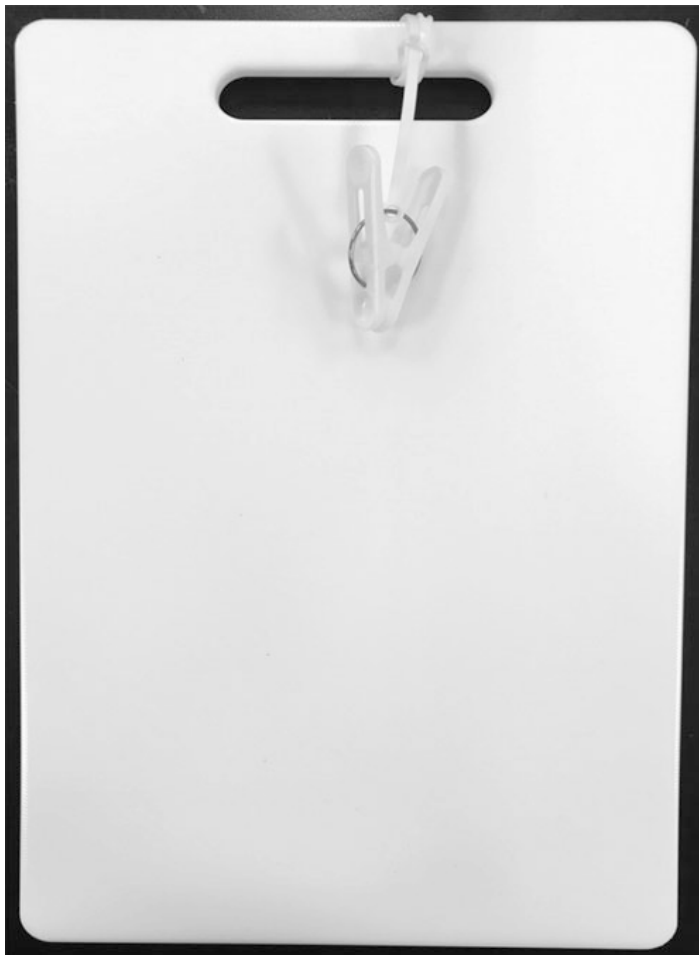
Fig. 1 A simplified holder for mouse. The holder consists of a chopping board and a clothing pin. The mouse is hold around the neck and its tail is pulled to apply a tension on its back
